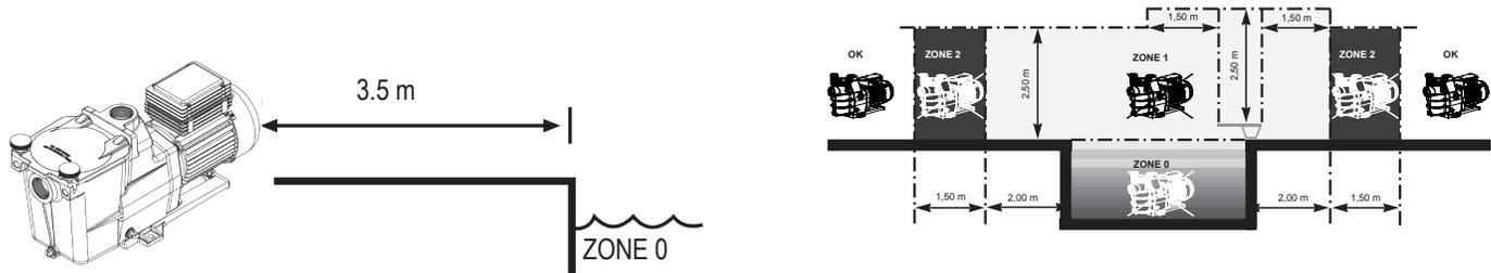
Install the pump in a dry, well-ventilated place. The motor requires the air to circulate freely around it to allow natural ventilation. Check regularly that no objects, leaves or other debris are blocking the motor cooling system.
