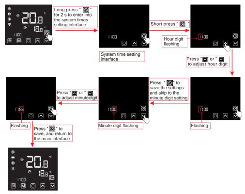
Notes: Under the clock setting interface, if there is no operation for 20 s, the system will automatically memorize use's settings, and return to the main interface; if short press uring any operating steps, the changes will not be saved and return to the main interface.
