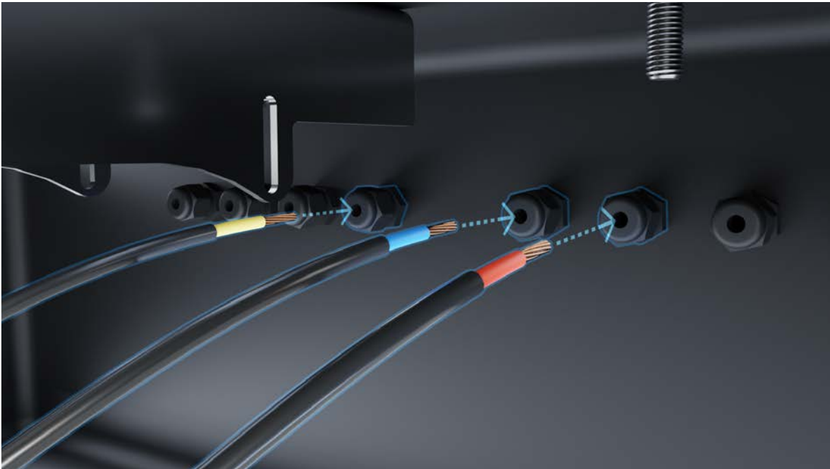
3. Put the turbine cables through cable glands Use red, orange and black cables. Do not change the colors of the cables!
